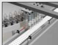
Clear plastic bottle detection (Detect presence/absence of bottle)
